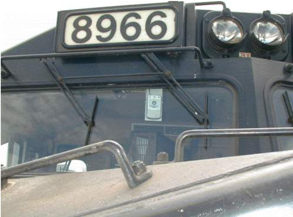
FIGURE 9 Norfolk Southern's RailView system features a camera mounted in the windshield of the locomotive's cab (Norfolk Southern 2003).
