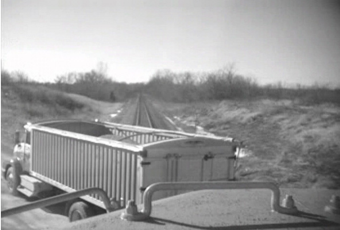
FIGURE 10 Image of a near collision at an HRGC taken from the camera of a Union Pacific TIR system (UPRR 2008).
